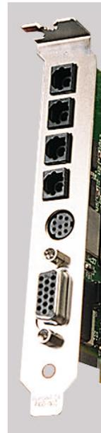
Any optical port can be switched from multichannel ADAT optical format to stereo SPDIF format for connectivity with DAT machines, MiniDisc recorders, or any other TOSLINK-compatible equipment.
