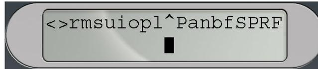
10. As you rotate the data wheel, the box will move left or right one character position with each tick of the data wheel, wrapping to the opposite edge of the display when moved past either edge. Move the data wheel clockwise and counter-clockwise, verifying that the box character moves right and left accordingly.
