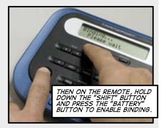
AFTER A COUPLE OF SECONDS, THE LINK LIGHTS ON BOTH UNITS SHOULD COME ON SOLID.
