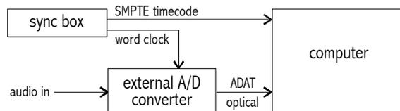
The sample rate (audio clock) in the ADAT optical signal and the frame rate (timecode) in the SMPTE signal must be locked together. Otherwise, the digital audio system doesn't know which rate to follow.
